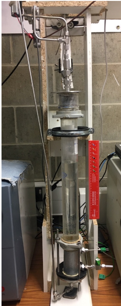
(a) Original prototype industrial reactor to track the permanent sequestering of CO 2 (g) by Mg(OH) 2 ; (b) Proposed initial design of flow cell for in situ neutron scattering observation of CO 2 mineralization at the (c) UK's neutron facility. (d) 3D model and Engineering Design Specification.
